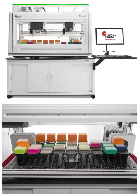
Figure 1. Biomek i7 DH Workstation with optional enclosure on a Biomek Mobile Workstation. Deck layout in the lower image.
