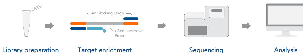
Figure 1. xGen target capture workflow. xGen Blocking Oligos bind to adapter sequences during target enrichment using xGen Lockdown Probes.
