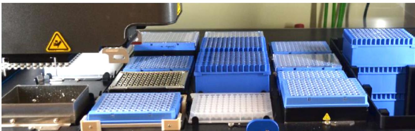
Figure 6. Deck layout for the Target Capture
