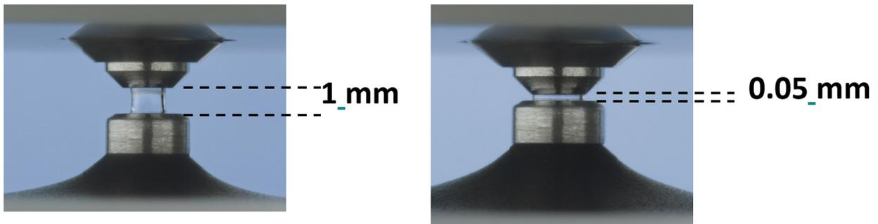
Figure 2. Path length affects error tolerance. The NanoDrop 2000 can take measurements at path lengths of 1–0.05 mm. This enables the instrument to measure a wide range of nucleic acid concentrations. It is important to realize that error tolerances for shorter path lengths are higher than those for longer path lengths.
