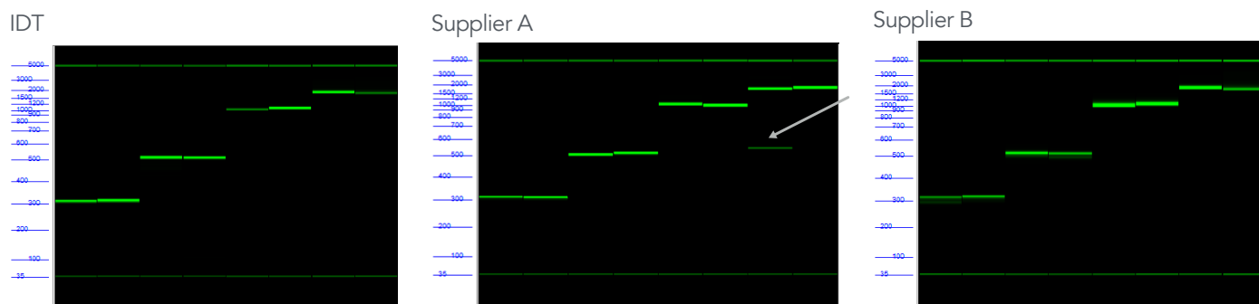
Figure 3. Another supplier's dsDNA fragments show the presence of truncated product in gel image output. Outputs from the Agilent fragment analyzer show strong bands from all suppliers, corresponding to the correct length on the ladder. However, in the sample from Supplier A, a second smaller band is seen, indicating the presence of a truncated product.
